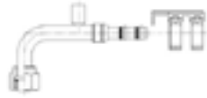
Female 90 Degree O-Ring with 13mm Switch or Service Port Fitting with Clamp
