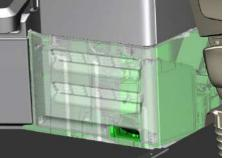
Dual HVAC System under the cabinet (evaporator, compressor, heater core, and blower)
