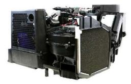
Condenser mounted on the exterior of the back sleeper with your choice of mounting location; either left or center. Below
